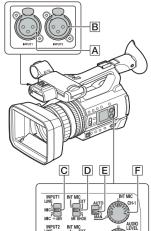
8) Press the GAIN button (E) to enable manual gain control for exposure. Try not go past 15db or things get pretty noisy.
